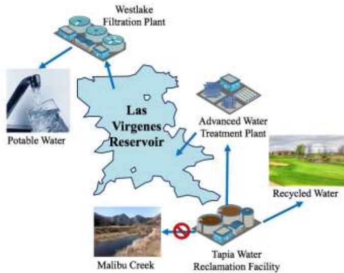
**Figure 1. Schematic of the Las Virgenes-Triunfo Pure Water Project (Credit: Trussell Technologies).**
